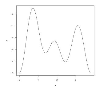
This structure is made of three atoms (three peaks), roughly located between 0 and 1, close to 2 and close to 3. In order to find out the correct location of the peaks, and thus the coordinates of the atoms, we make use of local\_maxima. The maxima and minima in the electron density are returned as integers corresponding to specific cells of the electron density array.
