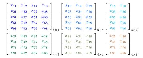
Figure 2: Local Processor Storage View of the Block Cyclic Data Decomposition
