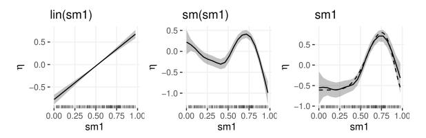
Figure 4: Posterior means and pointwise 80% credible intervals for  $f(\mathtt{sm1})$  in  $\mathtt{m1}$ . Left and middle panel show the separate  $\mathtt{lin}()$ - and  $\mathtt{sm}()$ -terms returned by the first call to  $\mathtt{plot}$ , right panel shows their sum. True shape of  $f(\mathtt{sm1})$  added as a dashed line with the  $\mathtt{ggElems}$  option of  $\mathtt{plot}.\mathtt{spikeSlabGAM}$ , see lines of code above the figure.
