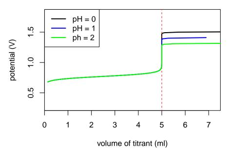
Note that the change in potential at the equivalence point decreases with an increase in pH because the potential for the titrant's half-reaction decreases with an increase in pH.
