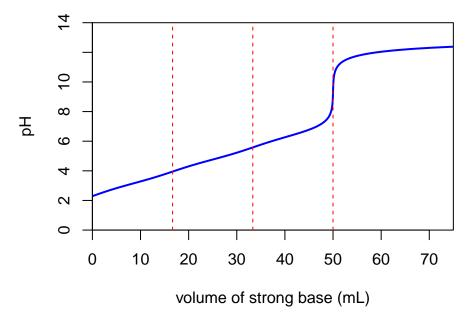
Note that because the first two  $pK_a$  values are not sufficiently different from each other, the titration curve shows just one distinct equivalence point for the titration of citric acid's third proton.
