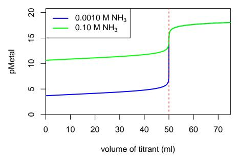
Note that the change in pM at the equivalence point is much greater for the smaller concentration of  $NH_3$ ; this is because a greater fraction of  $Cu^{2+}$  remains free from complexation before the equivalence point.
