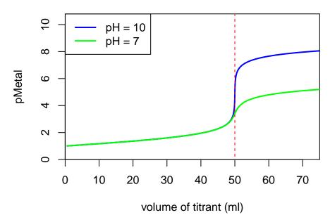
Note that the change in pM at the equivalence point is much greater at a pH of 10 because a greater fraction of the EDTA is in its fully unprotonated form at this pH.
