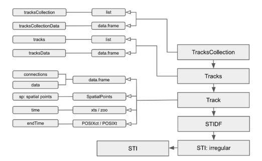
Figure 3: Classes for trajectory data in the package trajectories. Solid arrows denote inheritance. Arrows show the corresponding slot's class and slot's names are displayed using lines accordingly.
