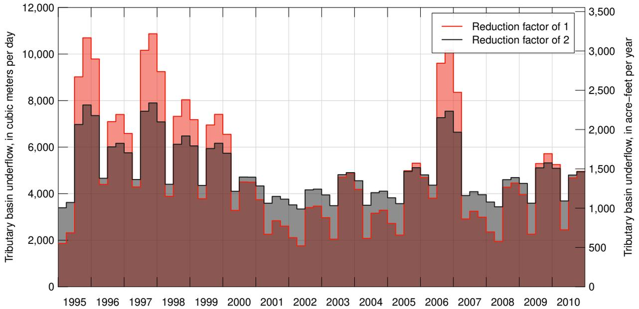
**Figure E7.** Seasonally adjusted tributary basin underflow in the Deer Creek tributary canyon calculated using a reduction factor of 1 and 2, while holding constant the sampling window at 9 months and estimated long-term average underflow at 4,937 cubic meters per day.
