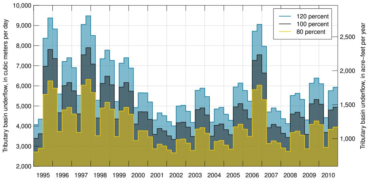
**Figure E8.** Seasonally adjusted tributary basin underflow in the Deer Creek tributary canyon calculated using 120, 100, and 80 percent of the estimated long-term average underflow (4,937 cubic meters per day). The sampling window and reduction factor were held constant at 9 months and 2, respectively.
