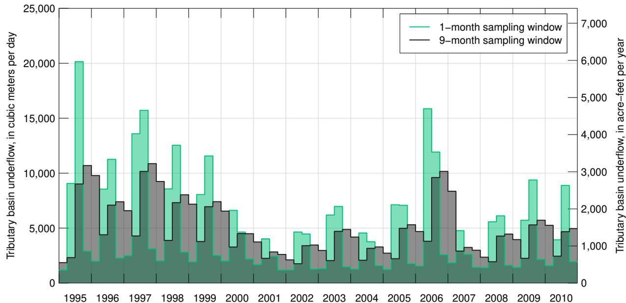
**Figure E6.** Seasonally adjusted tributary basin underflow in the Deer Creek tributary canyon calculated using a 1- and 9-month sampling window, while holding constant the reduction factor at 1 and estimated long-term average underflow at 4,937 cubic meters per day.
